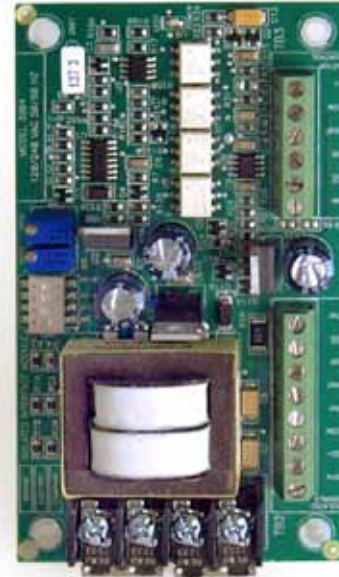
Model 3984 Analog Interface and Isolation Board for use with most basic chassis speed controls such as those shown below
